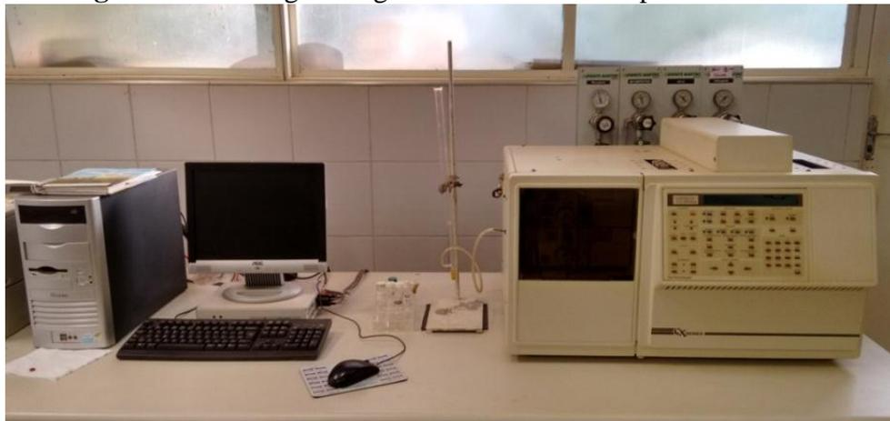
**Figura 6.** Analisador de Carbono Orgânico Total TOC-L
